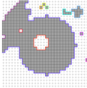
(b) Contour extraction in 2D using a topological cellular model
