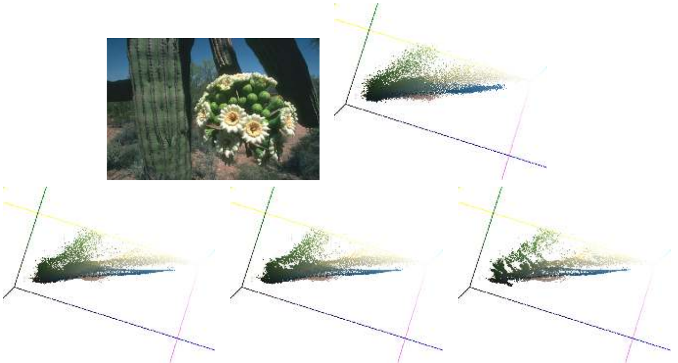
Figure 4: Top, original image and its color cube. The image is filtered with the LLP2 algorithm with T = 10 , \varepsilon = 0.5 and increasing values of the speed-up parameter \delta . Bottom, from left to right, resulting cubes with \delta = 0 (no acceleration), \delta = 5 and \delta = 10 . For large values of \delta (bottom-right) the filtered color clouds tend to be composed of unconnected 2D manifolds, instead of forming a smooth surface (bottom, left and center).
