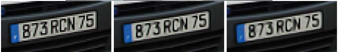
Figure 40: Top, original image. Bottom: left, 6× zoomed detail from original; center, MCM evolution at scale 2/3; right, AMSS evolution at scale 2/3.
