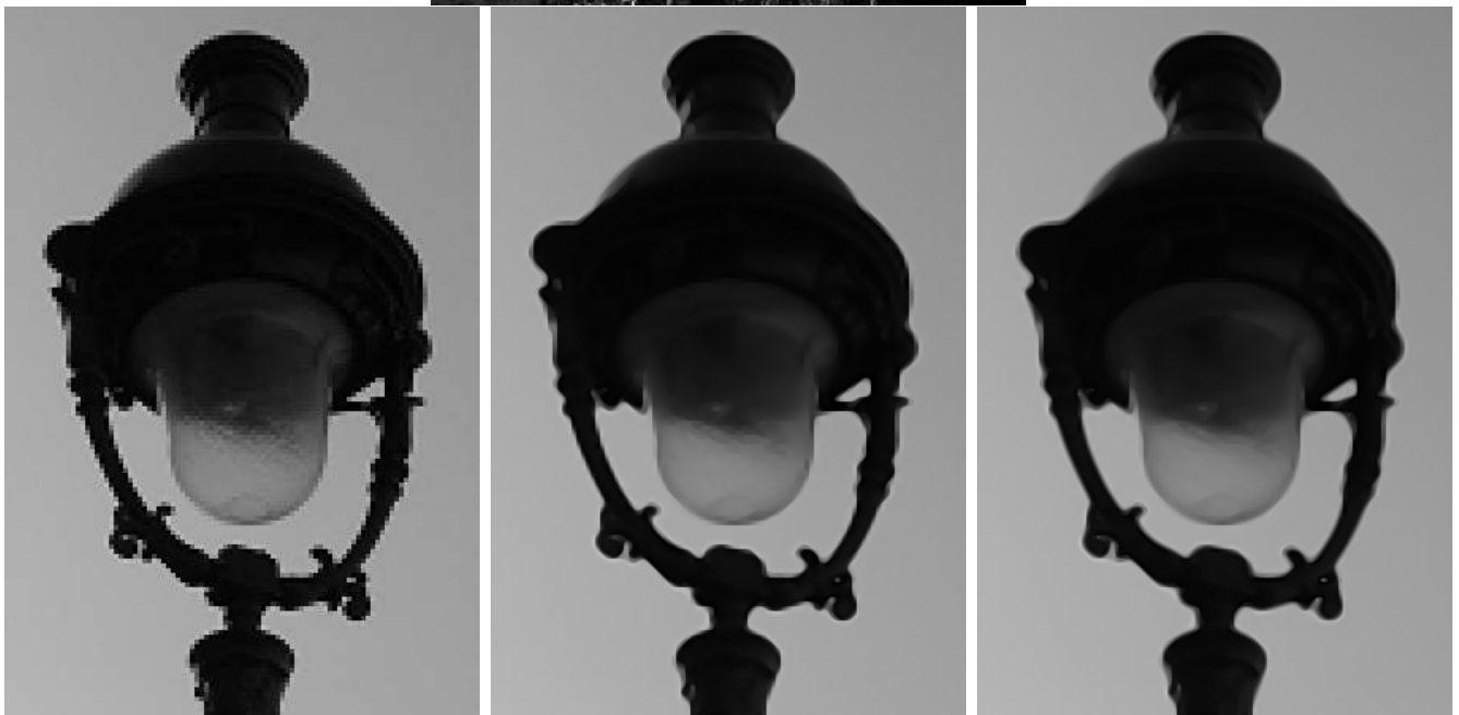
Figure 44: Top, original image. Bottom: left, 3× zoomed detail from original; center, MCM evolution at scale 5/6; right, AMSS evolution at scale 5/6.
