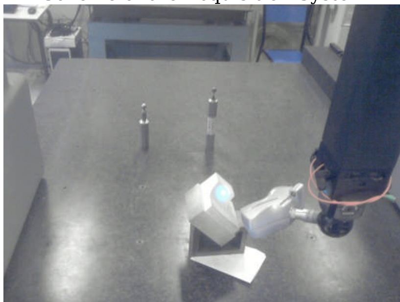
Laser ray projected on the surface of the object to digitize
