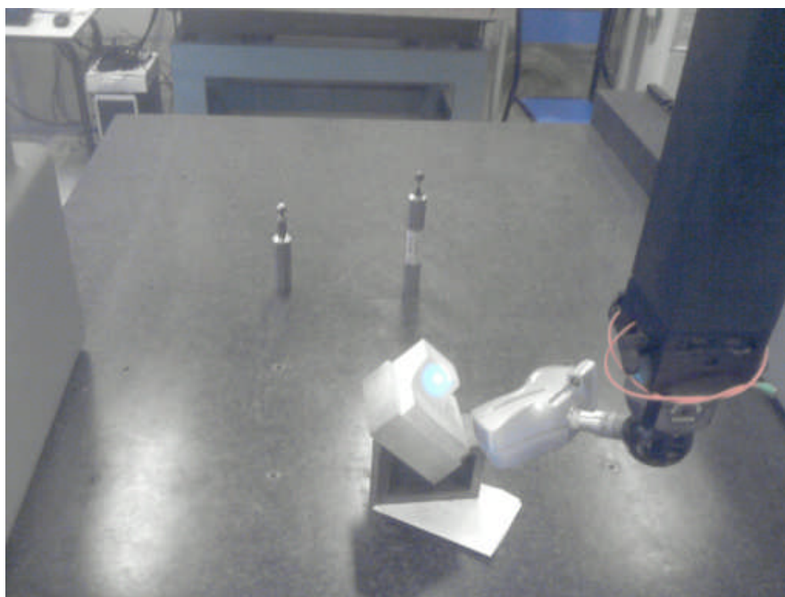
Figure 2: Laser ray projected on the surface of the object to digitize.
