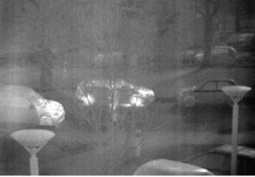
Figure 1: Observed image (left) taken with a *Thales Minie-D* camera, corrupted by a structured noise called *non-uniformity*. It comes from a non-uniform response of the readout system to the same amount of photons sensed. In the corrected image (right), the *non-uniformity* is much reduced.
