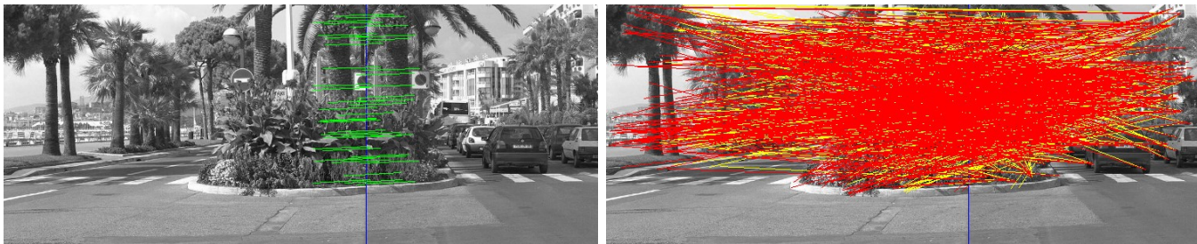
Figure 6: Registration of a crop of left Croisette image with right image, SIFT ratio s = 1 . Inliers ( 43/609=7\% ) and outliers ( 566/609=93\% )
