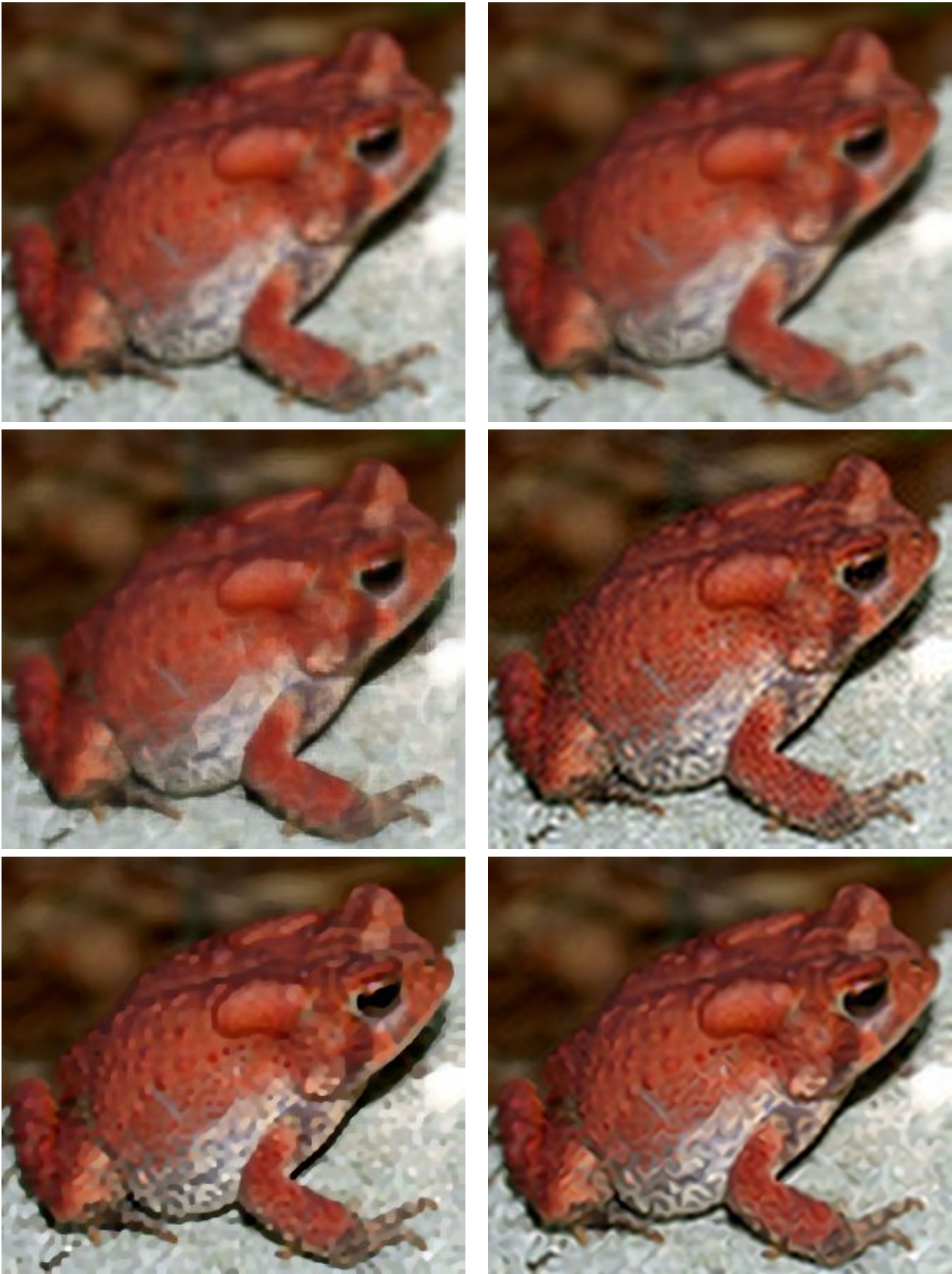
Figure 5: Interpolation results on the input image of Figure 4 for different methods. See text for details. From left to right and from top to bottom: Bicubic (PSNR 24.36, MSSIM 0.6311, CPU time 0.012s), AQua-2 (PSNR 23.97, MSSIM 0.6062, CPU time 0.016s), Fractal Zooming (PSNR 24.50, MSSIM 0.6317), Fourier Zero-Padding with Deconvolution (PSNR 25.70, MSSIM 0.7104, CPU time 0.049s), TV Minimization (PSNR 25.87, MSSIM 0.7181, CPU Time 2.72s), Tensor-Driven Diffusion (PSNR 26.00, MSSIM 0.7297, CPU Time 5.11s).
