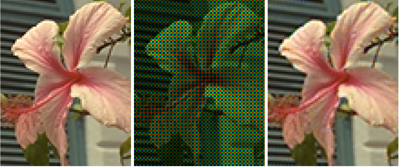
Figure 1: Example of demosaicking. Left, original image. Center, simulated image displaying the Bayer pattern. Right, demosaicking result of Malvar, He, and Cutler’s method, after processing the simulated image. The images are enlarged to show individual pixels more clearly.
