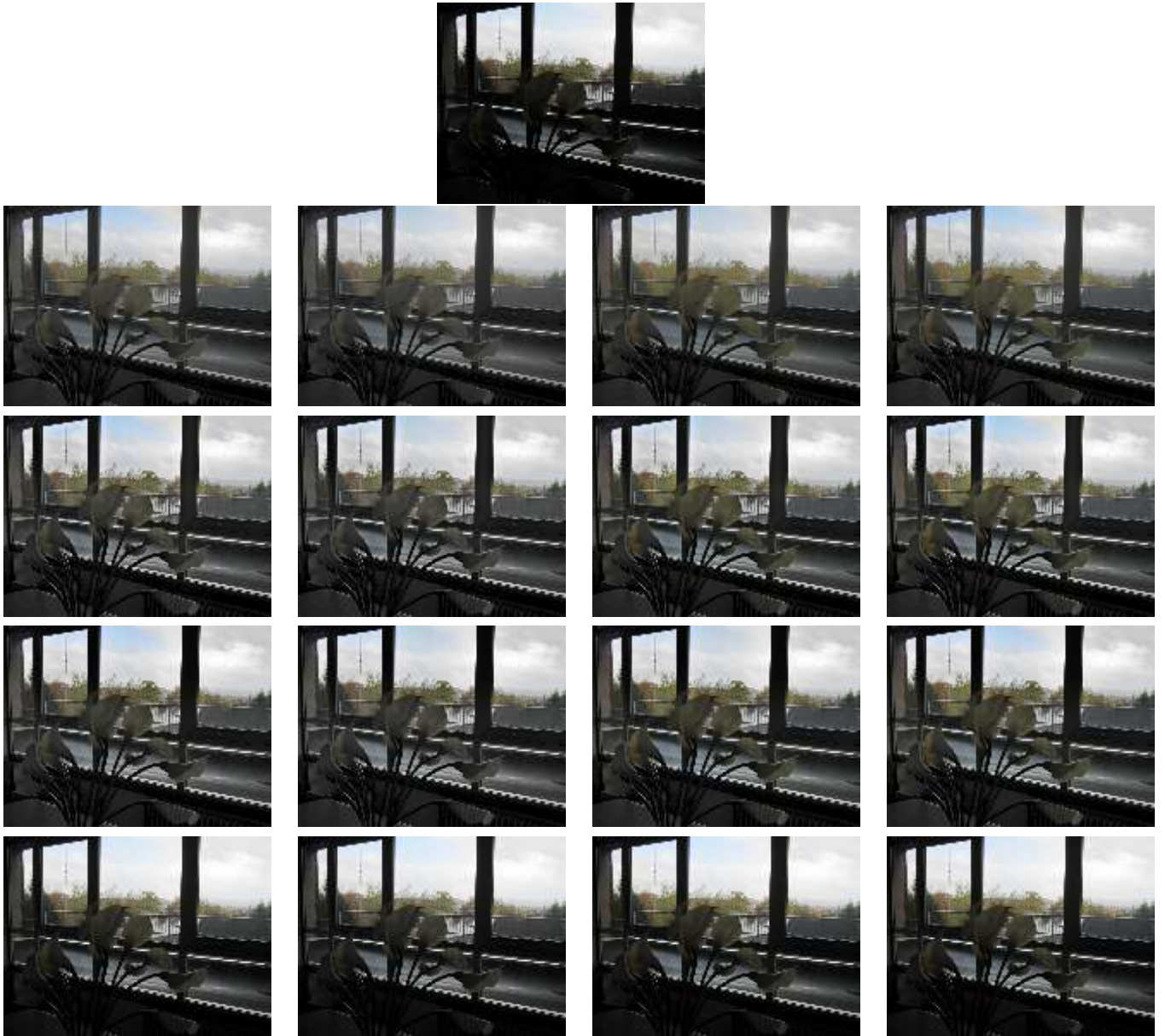
Figure 13: Top, original image. The subsequent rows display (from left to right) the results of LCC-RGB, LCC-YPbPr, LCC-HSI, LCC-HSL for increasing values of the parameter r . From top to bottom, r = 0 , r = 40 , r = 100 . The last row displays the result of global gamma correction with default \gamma value as defined by (6).
