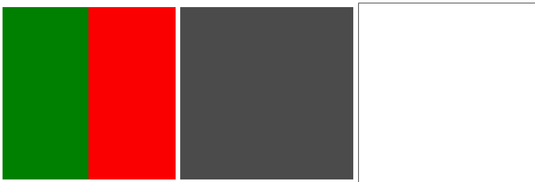
Figure 23: Color , 254 \times 254 pixels. LSD is designed to work on gray-level images. Before applying LSD to a color image it must be converted to a gray-level image. However, some color edges could be lost in this conversion. For example, the image on the left presents a clear edge, but after the standard conversion to a gray-level image (middle) the edge is lost. The reason is that the red value and the green value are both converted to the same gray value. Thus, LSD will produce no detection (right) because none is present in the input image to LSD (middle). The edge is lost on the color to gray image conversion and not by LSD. An extension of LSD to deal with this (relatively rare) event is possible but was not done in the current implementation.
