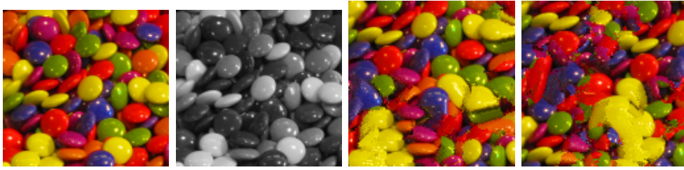
Figure 13: Reproducibility of results. From left to right: sample image, gray level version, result obtained using the classical implementation of [8], result obtained using the accelerated implementation. Some candies having different colors in the sample image are merged in the gray level version corresponding to the first component of the PCA. Color artifacts appear when using the accelerated implementation. This case is quite uncommon.
