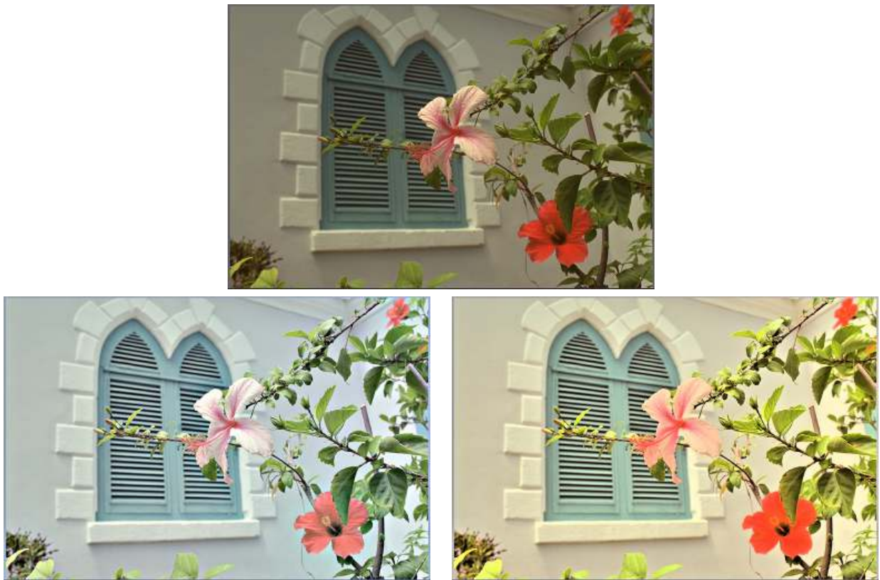
Figure 10: Top: Original image. Bottom left: Result of MSRCR. Bottom right: Result of MSRCP.
