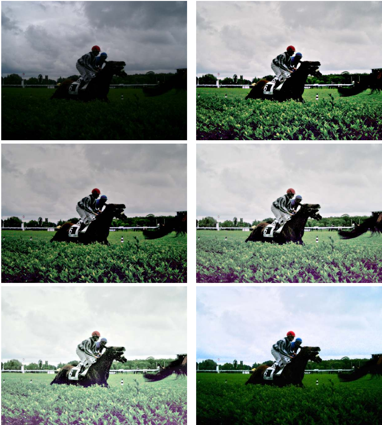
Figure 5: Comparison of different gain/offset. Top Left: original image. Top right: result of the original MSRCR with G = 30 and b = -6 . Center left: result with G = 25 and b = -6 . Center right: result with G = 20 and b = -10 . Bottom left: result with our version using the simplest color balance, with 1% of saturation, as postprocessing, that is, result of MSRCR algorithm. Bottom right: result with simplest color balance, with 1% of saturation, on the intensity channel, that is, result of MSRCR algorithm.
