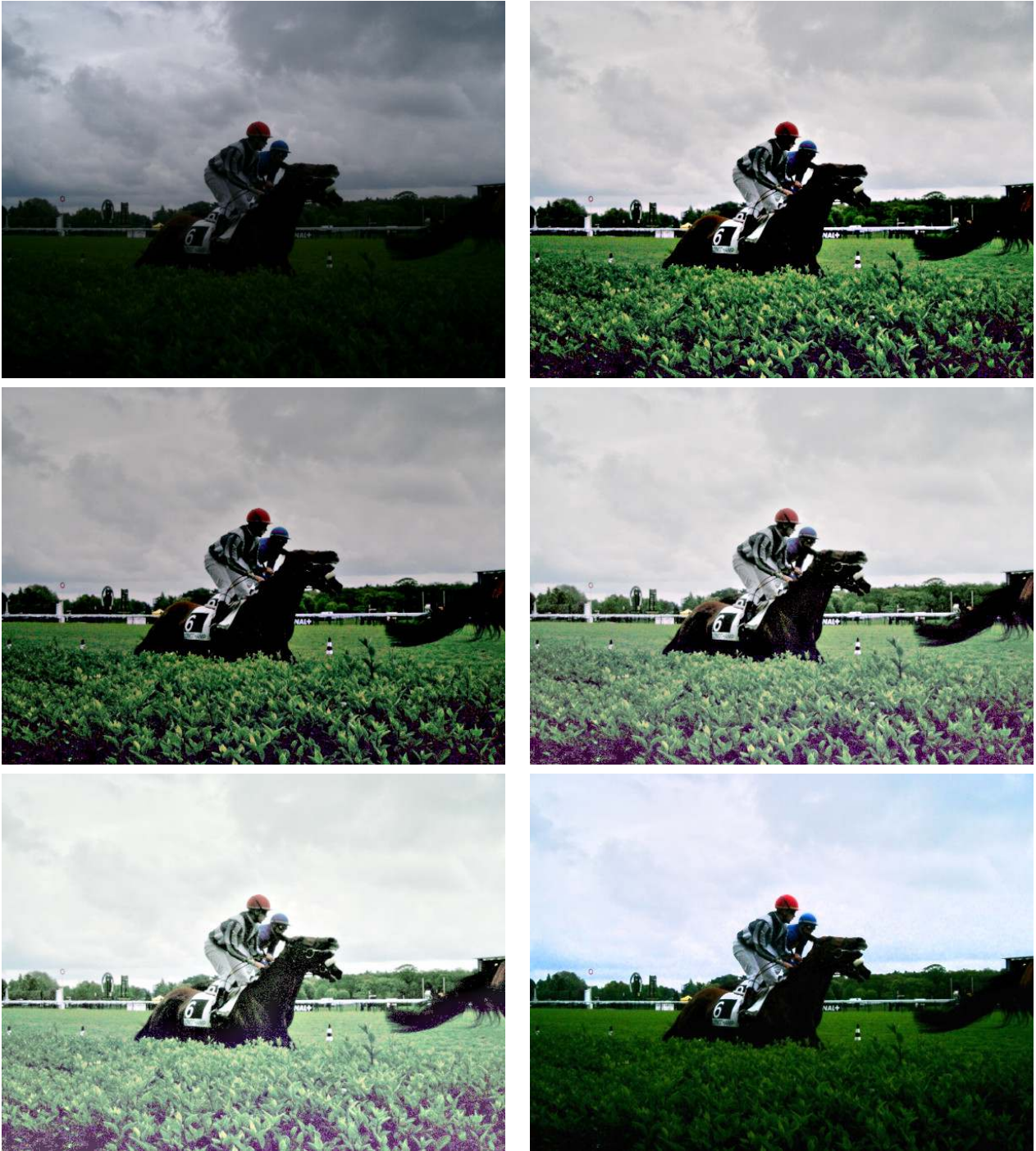
Figure 5: Comparison of different gain/offset. Top Left: original image. Top right: result of the original MSRCR with G = 30 and b = -6 . Center left: result with G = 25 and b = -6 . Center right: result with G = 20 and b = -10 . Bottom left: result with our version using the simplest color balance, with 1% of saturation, as postprocessing, that is, result of MSRCR algorithm. Bottom right: result with simplest color balance, with 1% of saturation, on the intensity channel, that is, result of MSRCP algorithm.
