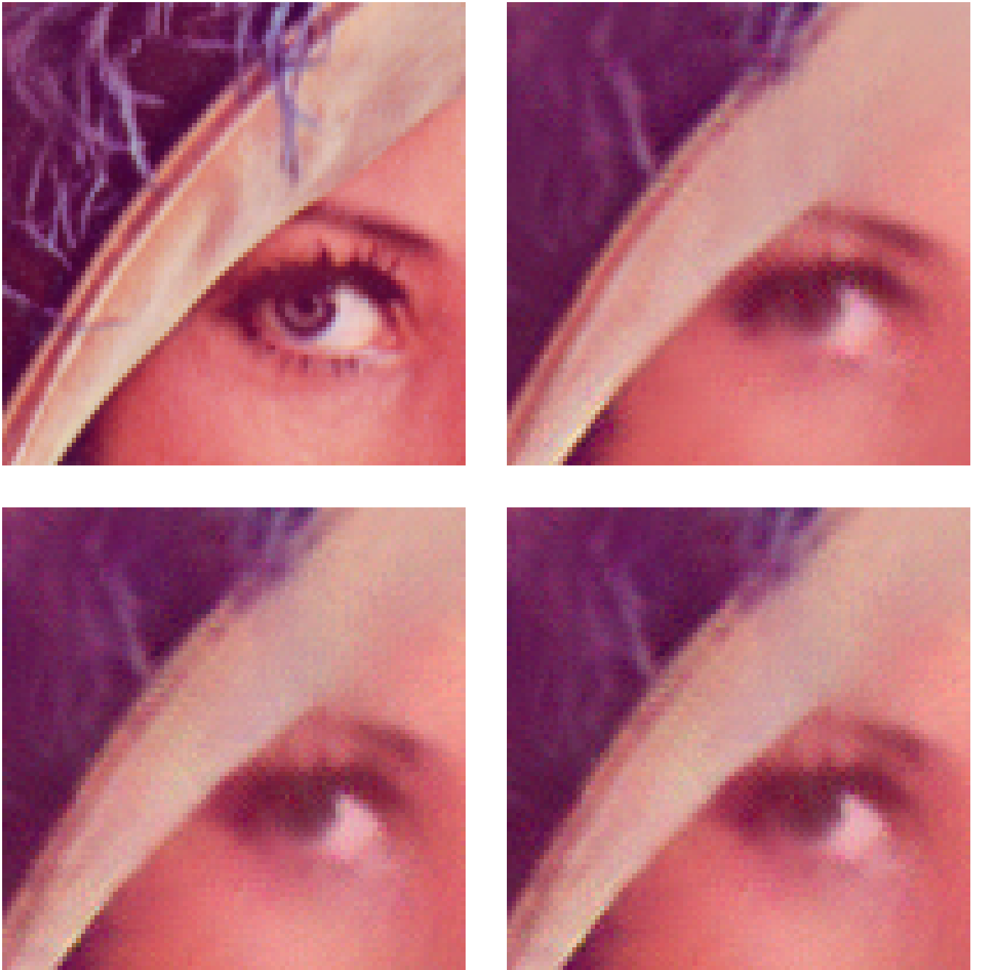
Figure 8: Visual comparison of parameter-free denoising algorithms applied on Lena image ( \sigma = 60 ; zoom on a part but PSNRs are computed on the whole image; in this experiment the noise realization is the same for all of the three denoising algorithms). From left to right and top to bottom: original u ; NLM-B (PSNR=27.18); NLM-P (PSNR=26.43); NLM-Pa (PSNR=26.43).
