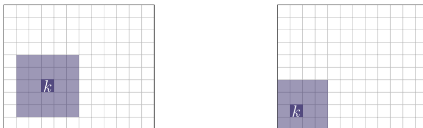
(a) Window of radius r_{\text{GF}} = 2 centered at k = (3, 6) . |\omega_k| = 25 .
