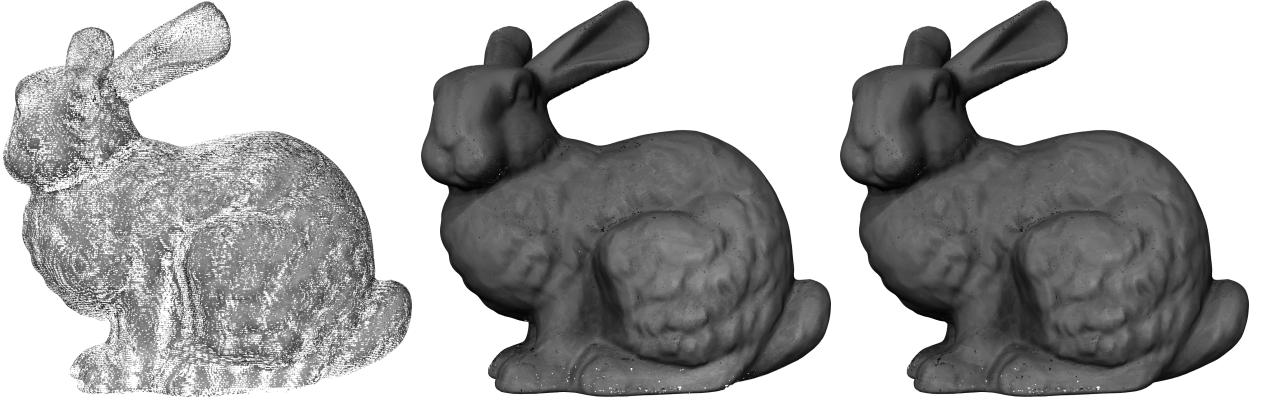
Figure 5: Limitations for the Ball Pivoting Algorithm: detail loss and hole creation due to a too large radius (left) and a too small one (middle). A possible solution is to use multiple radii (right): here three different radii are used successively from smallest radius to largest one, allowing for the recovery of details and the filling of the holes.
