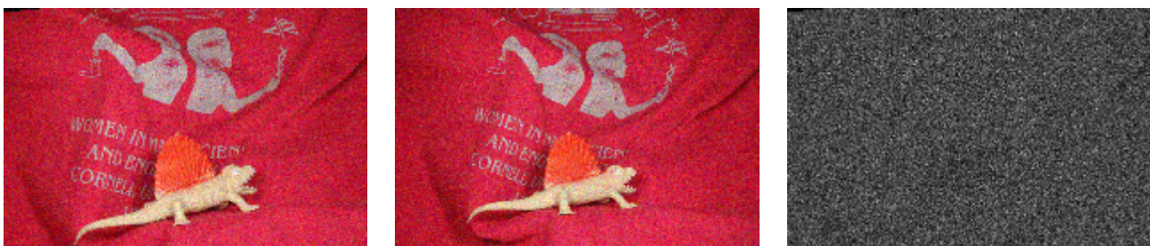
Figure 7: Two images of the Dimetrodon sequence related by a similarity, with Gaussian noise of \sigma := 20 . On the right, the error image given by |\mathbf{I}_2(\mathbf{x}'(\mathbf{x}; \mathbf{p})) - \mathbf{I}_1(\mathbf{x})| at each pixel.
