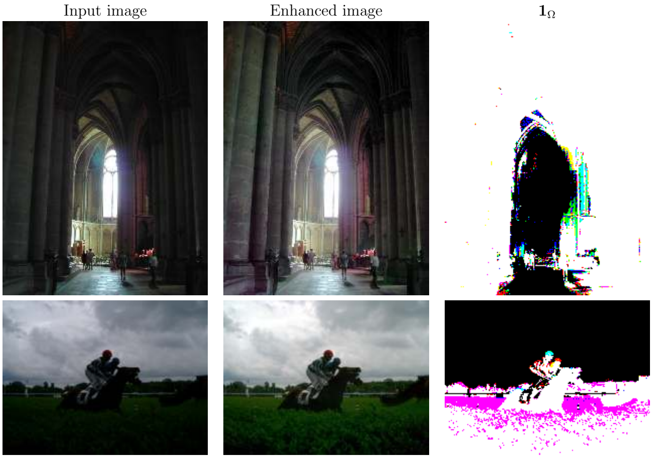
Figure 15: Contrast enhancement results obtained using the Finite differences numerical method . The region \Omega is computed for each color channel independently. In the third column the images display the red, green and blue components of \Omega .
