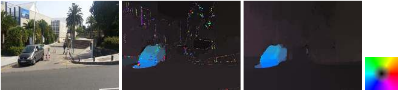
Figure 1: From left to right: The original image; instabilities over the computed flow field due to a wrong parameter; well-defined motion contours using our automatic strategy; the color scheme used for motion representation.
