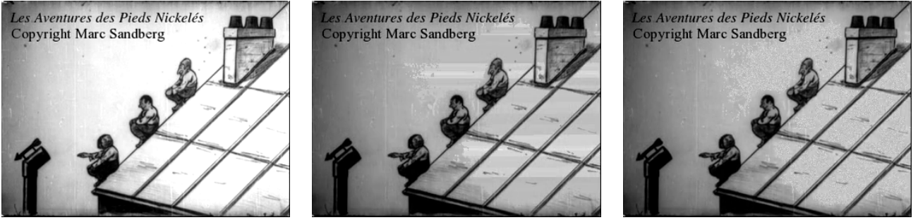
Figure 1: Artifacts appearing with the sorting method: On the left, one frame of the Pieds Nickelés sequence (see experiment in Figure 4); in the middle, the result of the sorting method without randomizing the gray levels (observe the strips of constant intensities); on the right, the result using the randomization.
