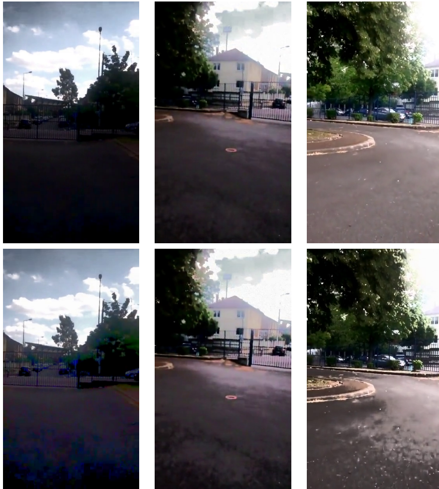
Figure 11: Equalization of the Walking sequence: Top row, equalization with the sorting method and \sigma := 30 ; bottom row, equalization with the same method and \sigma := 100 . We observe similar artifacts as in the histogram method (see Figure 10).
