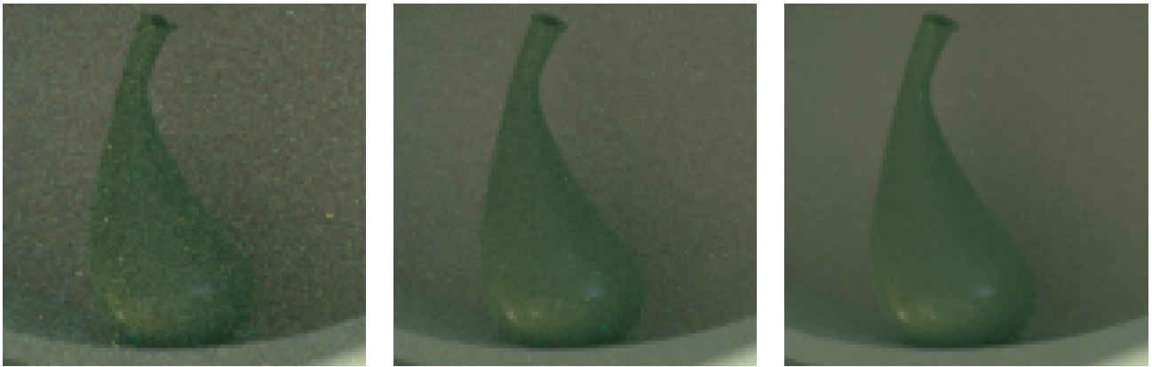
Figure 3: Example of residual noise in a shaded portion of the scene made for different durations. From left to right, the images were generated respectively for the periods T = 1 , T = 4 and T = 16 . Between two successive images the noise standard deviation is divided by a factor of 2.
