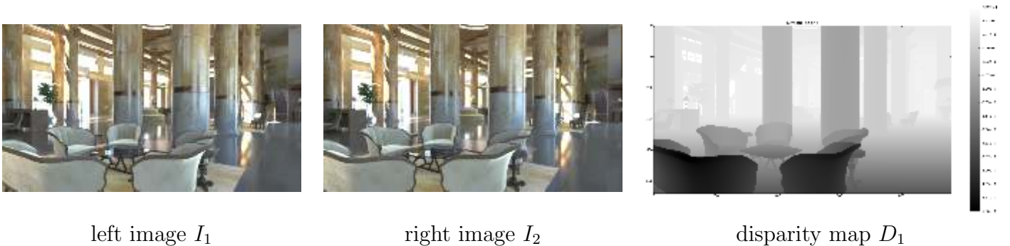
Figure 6: Example of disparity map obtained with a stereo pair (I_1, I_2) for which the camera made a maximal fronto-parallel displacement of 50 pixels.
