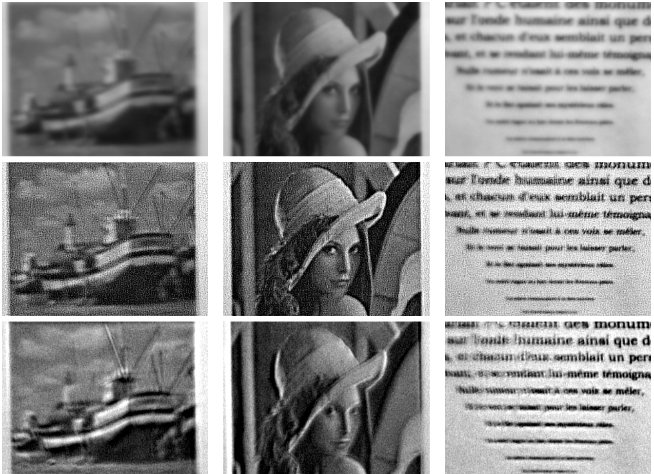
Figure 5: Results of experiment 1 applied on sequences at 5m of dataset A with M = 10 and \epsilon = 40 . From top to bottom: \mu the average of 10 images, L computed with the Laplacian filter, J computed with the SPCA filter.
