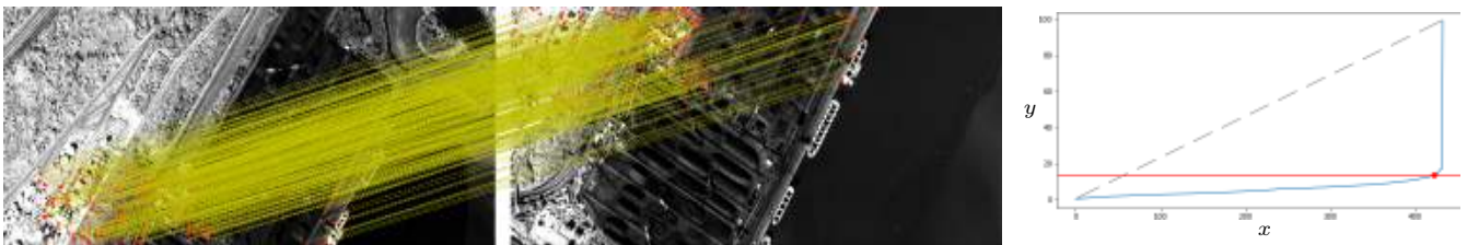
Figure 4: Example of pairwise matching result. The plot on the right shows, in blue, the sorted approximated geographic distances d_{\text{geo}} ( y -axis) for each match of a stereo pair ( x -axis), computed using (6). An outlier rejection threshold \tau , in red, is automatically set using the elbow point. The elbow point is defined as the point with largest distance with respect to the dashed line, i.e. the line defined by those points of the distribution with the minimum and maximum y values.
