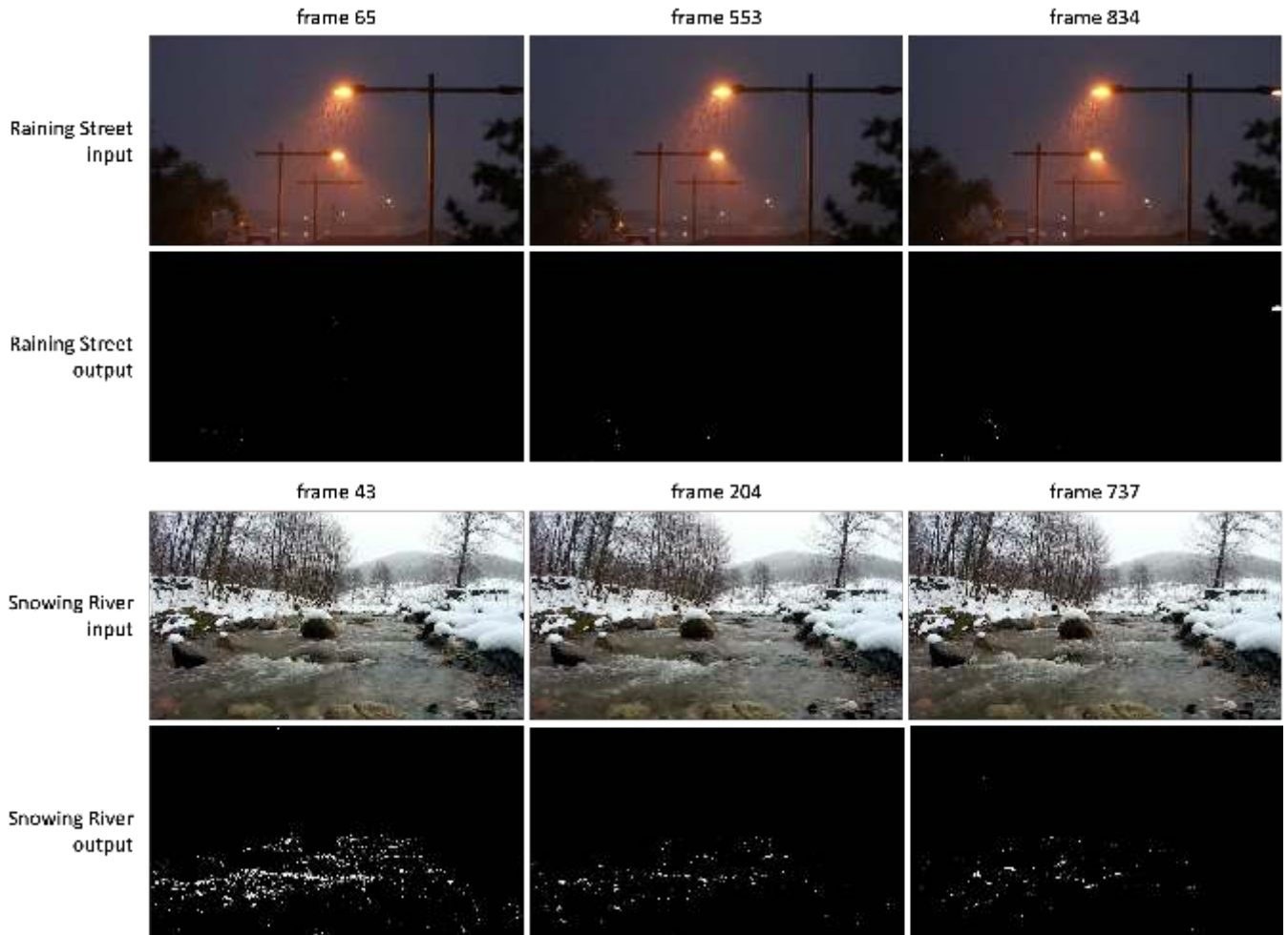
Figure 7: Results of ViBe for a set of frames of the two sequences involving bad weather and dynamic backgrounds.
