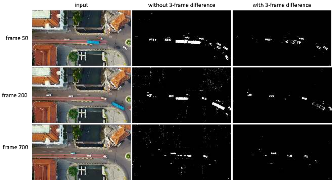
Figure 12: Illustrative example of the effect of the 3-frame difference variant to quickly dissipate ghosts, for three frames of the aerial street view sequence.
