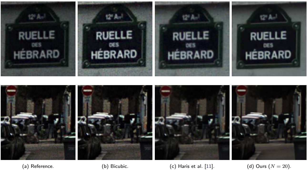
Figure 10: Comparison of different methods for \times 2 zoom on a real burst from [15]. The images are demosaicked using [10] and upscaled using several methods. Our pipeline manages to accurately recover the shape of the letters while removing the image noise. Better seen by zooming on a computer screen.
