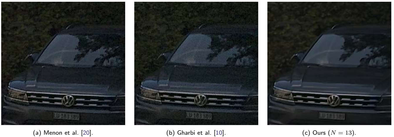
Figure 8: Quantitative demosaicking comparison. Our methods generates a sharp and noise free image. The licence plate is better demosaicked in our case, revealing all the numbers.
