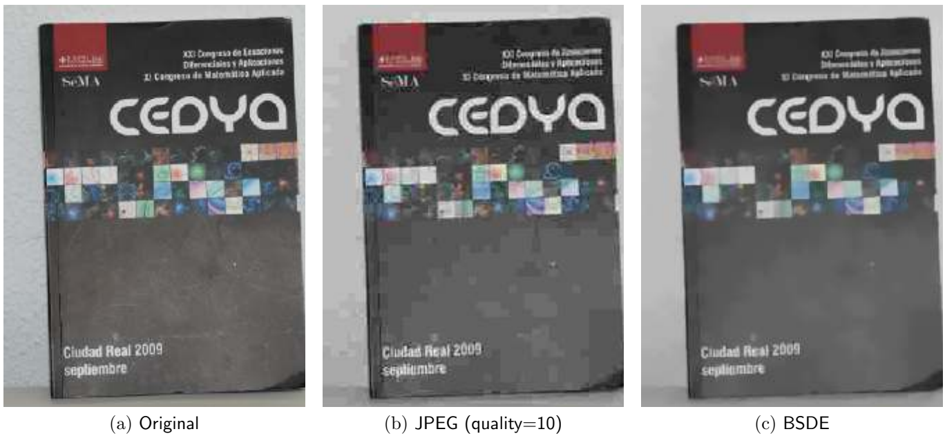
Figure 14: Reduction of JPEG artifacts. The BSDE algorithm was applied with \sigma = 17 and c = 0.0 .
