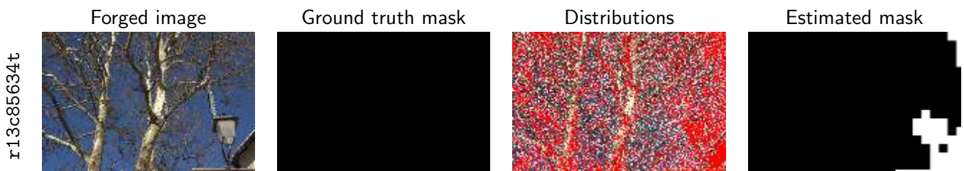
Figure 9: Example of false detection from the Trace dataset [3]. The image is highly textured. The method detects the flat zones in the image as forgeries.
