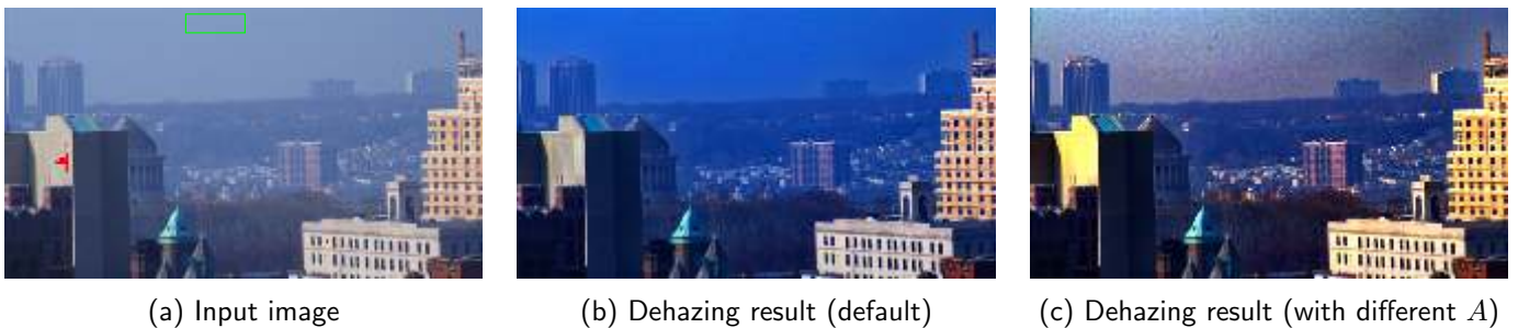
Figure 5: Effect of the ambient light estimation A on the result. In this image, the pixels used by default for the ambient light estimation are located on a bright building close to the camera. These pixels are marked in red in image (a). The corresponding dehazed image is shown in (b). Note the blue color cast of the image. On the other hand, using the pixels inside the green rectangle, displayed in (a), the ambient light is correctly estimated, leading to a result that doesn't exhibit the blue cast (c).
