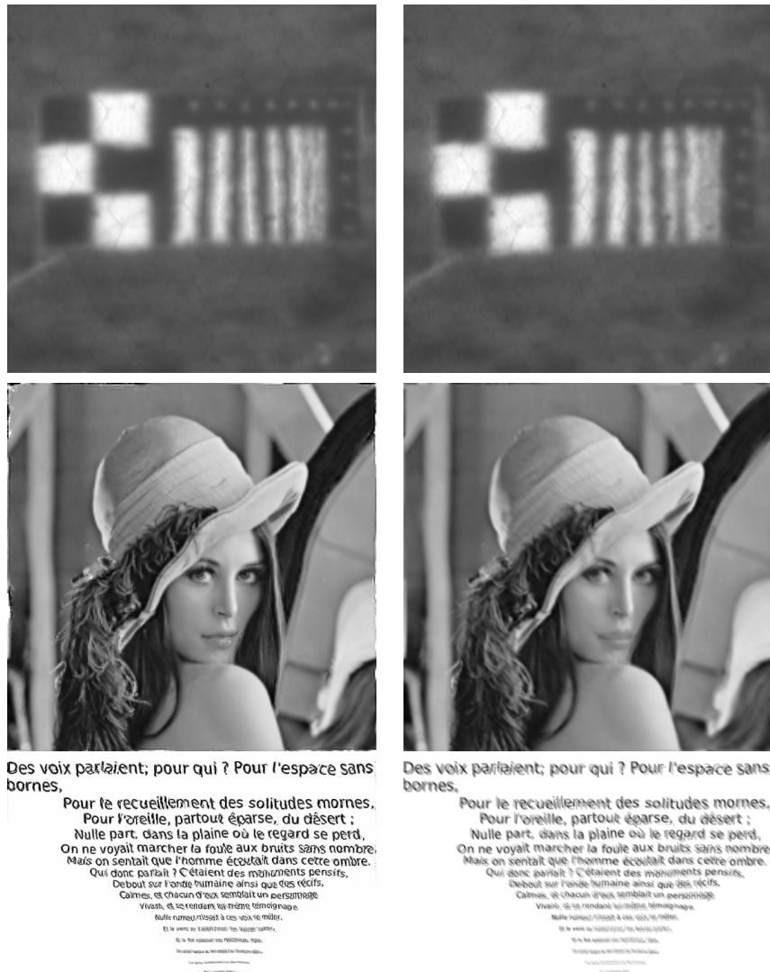
Figure 4: Stabilized (left) and temporal average (right) images obtained from the bars , lena and poème sequences, respectively.
