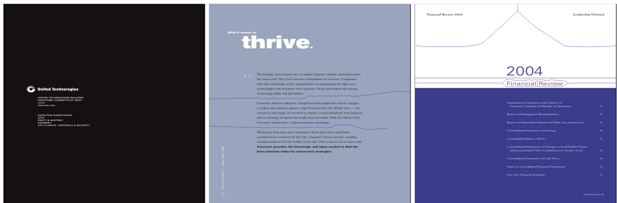
Figure 12: Results on documents with dark backgrounds and light-colored text. The binarization step in the current implementation assumes that background pixels are lighter than foreground ones. Therefore, the segmentation results in these examples are unsatisfactory.
