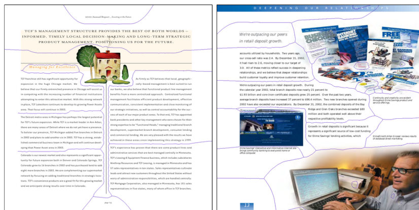
Figure 14: Results on non-Manhattan documents. In both examples, the irregular boundaries of the text surrounding the figures are correctly managed.
