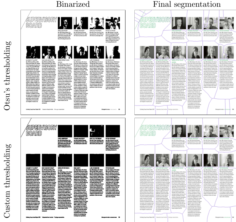
Figure 4: Comparison between Otsu’s thresholding and custom thresholding. When binarization is performed using Otsu’s threshold, parts of the pictures in the document are taken as background, causing an incorrect segmentation of those parts. A custom threshold set to 250 prevents such behavior and outputs correct region borders. The results shown here are obtained by setting N = 4 , w = 2 , \rho = 0.4 and T_A = 40 .
