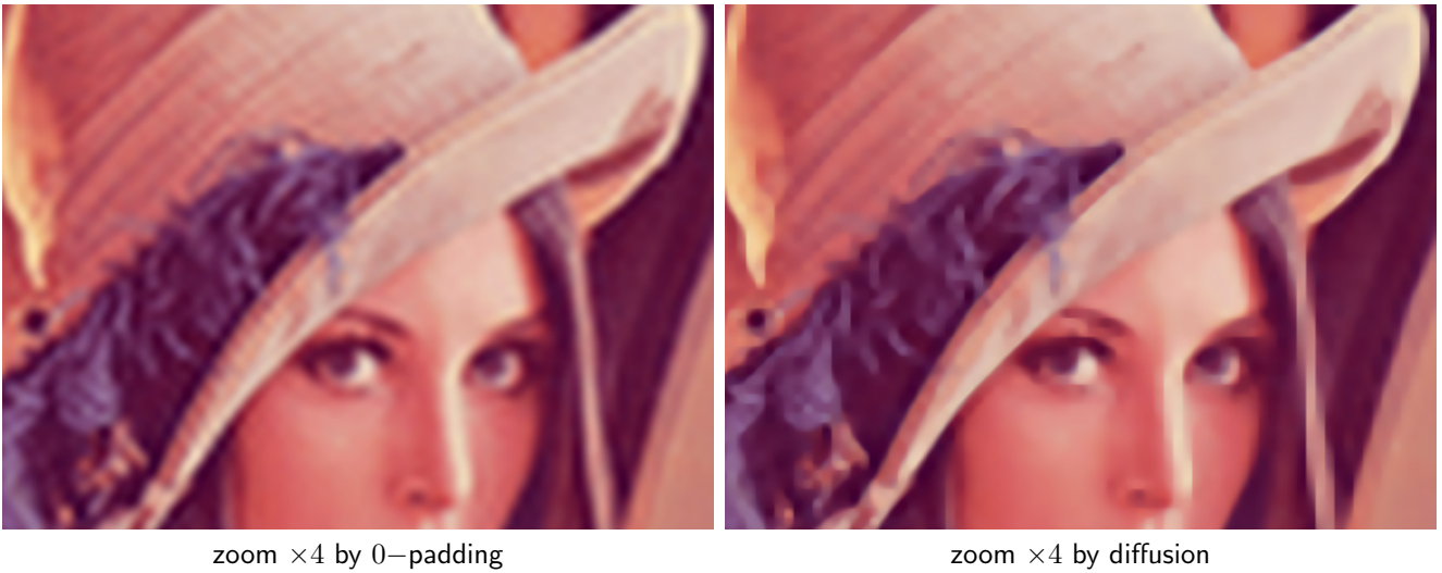
Figure 4: Super-resolution by 0-padding and by anisotropic diffusion.. Notice the ringing at the fringe of the hat, attenuated by the diffusion.
