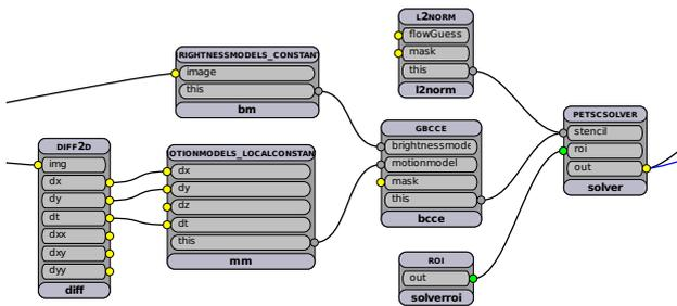
Figure 3: Example workflow showing the central part of our modular implementation of the algorithm by Horn & Schunck (1981). For simplicity, the modules reading the image data (at the left) and writing the flow result to a file (at the right) have been omitted. The visualization has been generated using the *tuchulcha* configuration and visualization tool.
