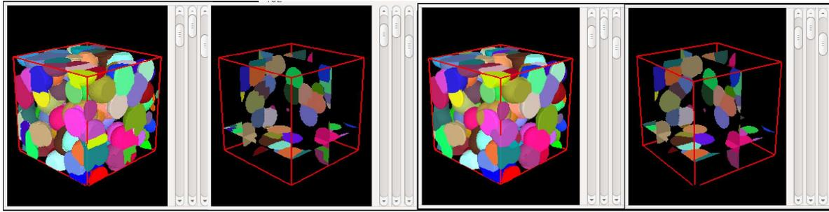
Figure 1: left figure: decomposition in elementary components with L. Vincent's procedure, right figure: regularization of the previous decomposition with Allen-Cahn equation for a minimal surface criteria
