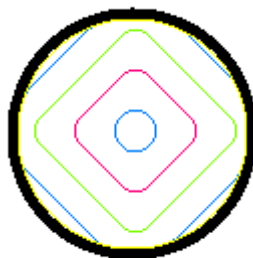
Ballon snake (type 2): Expand the original contour while the grey level is similar.
