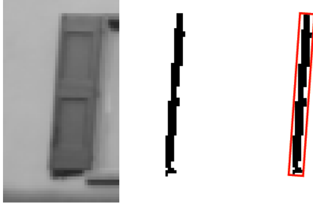
Figure 3: Rectangle approximation of line support region.
