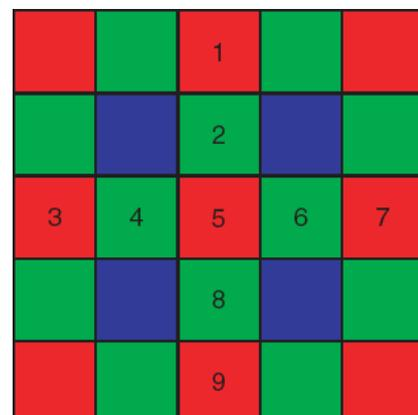
The red and blue channels are interpolated taking into account the already filled green channel. A bilinear interpolation is applied to the differences R-G and B-G as originally proposed by Cok [2].
