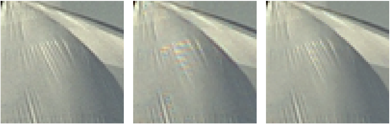
Figure 2: Original image (left) and demosaicking results of Hamilton-Adams algorithm (center) and SSD (right).
