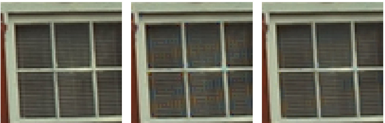
Figure 3: Original image (left) and demosaicking results of Hamilton-Adams algorithm (center) and SSD (right).
