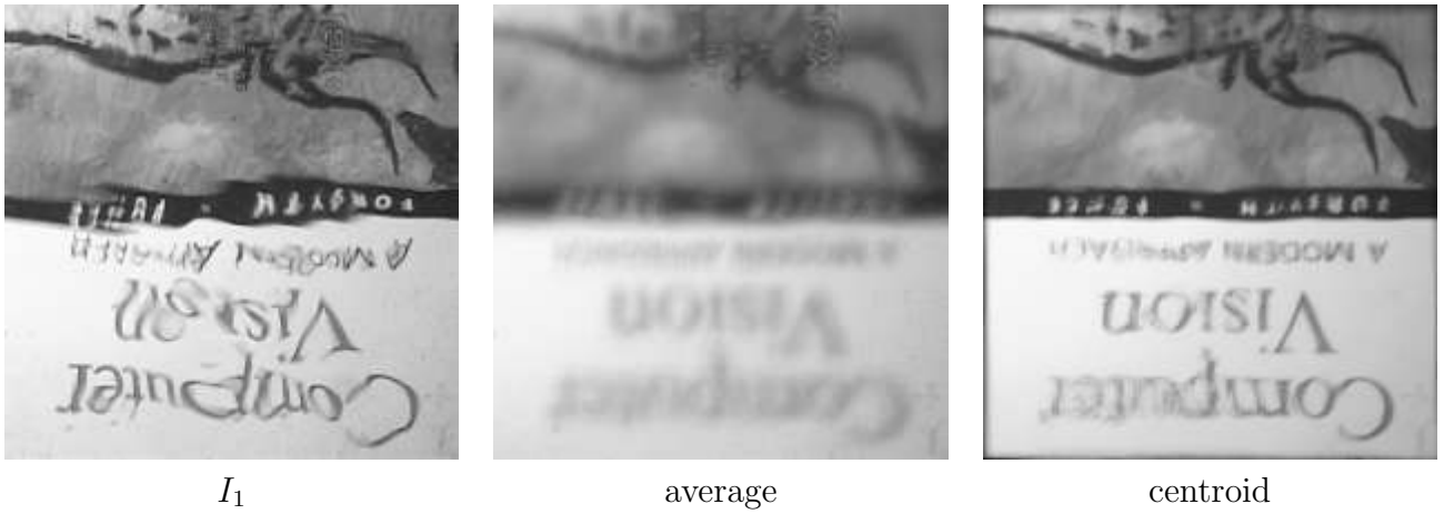
Figure 3: Result of the centroid method for the sequence from reference [4] (used with permission). This is an extract of 400 frames from the original sequence, cropped around the center of the image.
