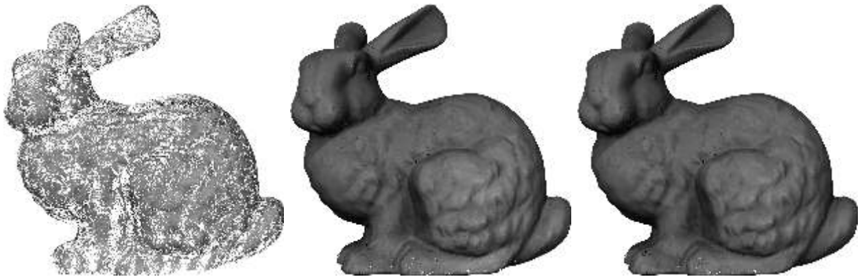
Figure 6: Reconstructing the Stanford Bunny point cloud, with a single radius (0.0003), two radii (0.0003; 0.0005) and three radii (0.0003; 0.0005; 0.002).
