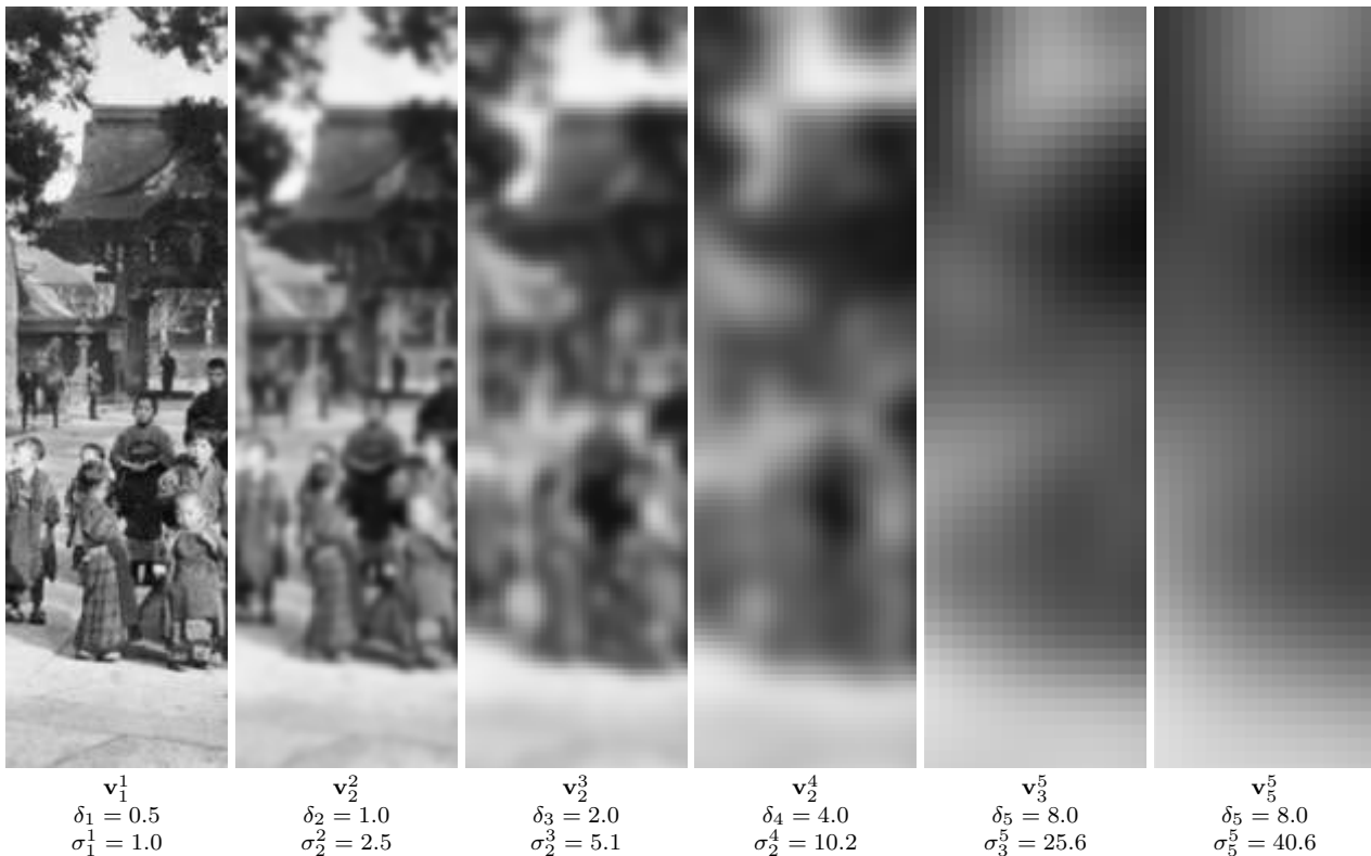
Figure 3: Crops of a subset of images extracted from the Gaussian scale-space of an example image. The scale-space parameters are set to n_{\text{spo}} = 3 , \sigma_{\text{min}} = 0.8 , and the assumed input image blur level \sigma_{\text{in}} = 0.5 . Image pixels are represented by a square of side \delta_o for better visualization.
