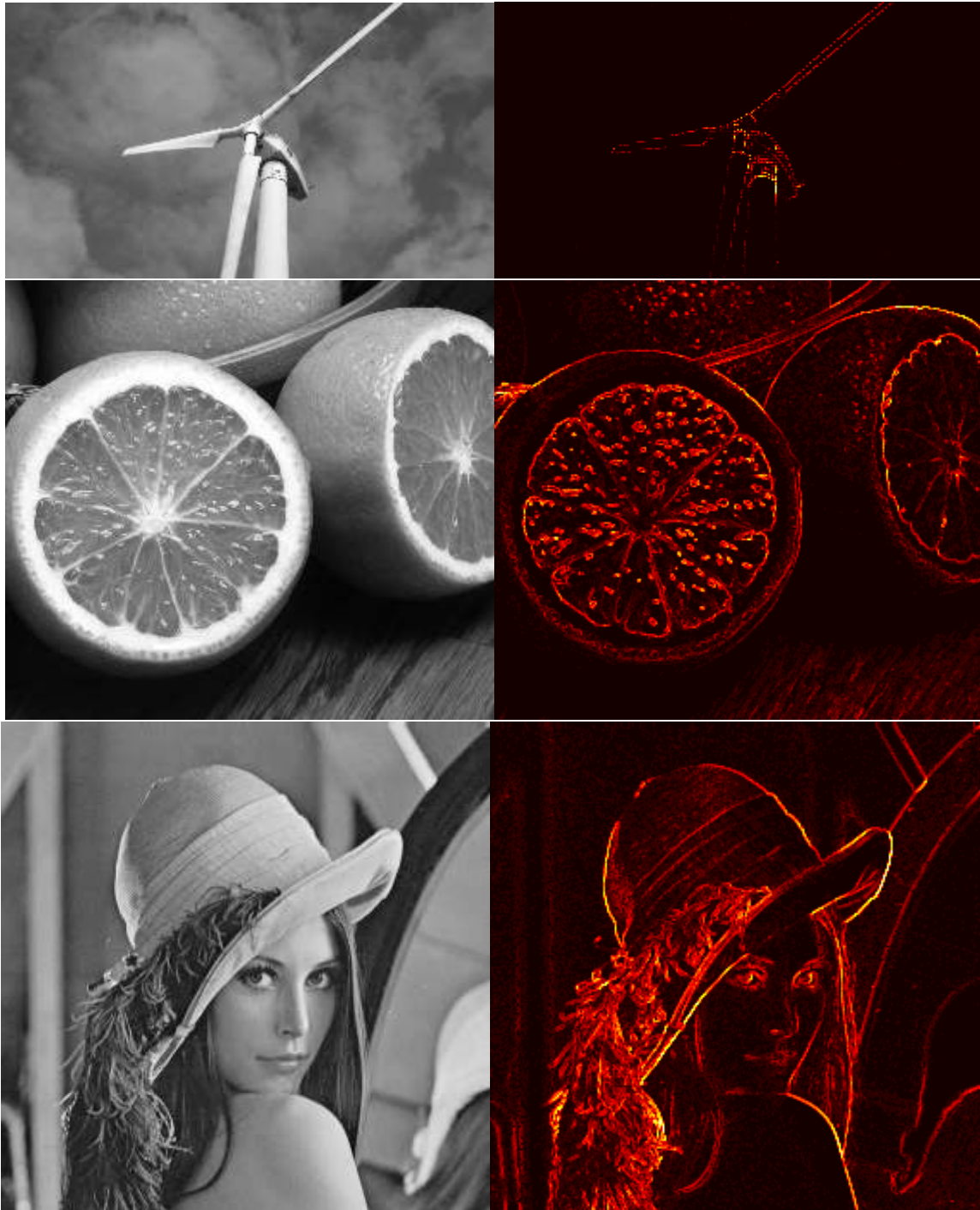
Figure 19: Results of the Roberts algorithm on our sample images. For each example we show the original image on the left and a saliency map on the right. The value of each contour corresponds to the scale of disappearance \alpha^- of each region.
