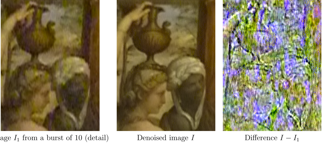
Figure 11: Example of burst denoising. These images show details of larger images of size 1920 \times 1080 . Notice that, besides being denoised, the reconstructed image is sharper. This is due to the weights used in the denoising, which tend to reject images in the burst which are blurry. The difference is shown here within the range [-20, 20] .
