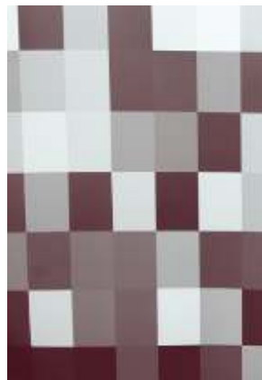
Figure 6: One of the pictures of the calibration pattern used to build the ground truth noise curve of the camera.
