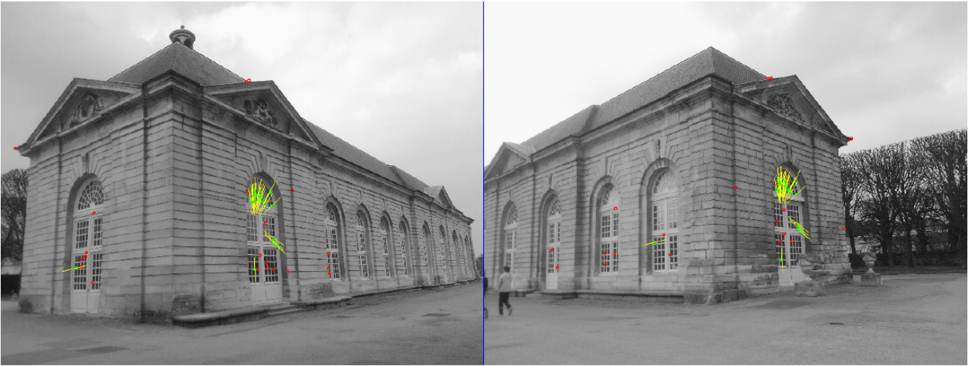
Figure 8: Incorrect estimated model between different façades of the Orangerie de Sceaux, with a threshold of 1.1 pixel.
