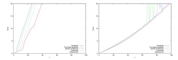
Figure 6: Linear parameter noise: Error evolution,  $\tilde{d}(\mathbf{H}_{gt}\mathbf{x}_i, \mathbf{H}_e\mathbf{x}_i)$ , with respect to Gaussian noise in the parameters. The transformations are calculated by linear interpolation between an initial set of points and points with Gaussian noise of  $\sigma := 50$ . Left graphic without the coarse–to–fine approach and, right, with four scales.
