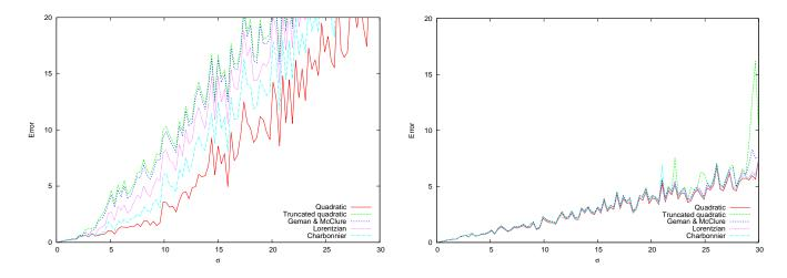
Figure 5: Parameter noise: Error evolution,  $\tilde{d}(\mathbf{H}_{gt}\mathbf{x}_i, \mathbf{H}_e\mathbf{x}_i)$ , with respect to Gaussian noise in the parameters. Left graphic without the coarse–to–fine approach and, right, with four scales.
