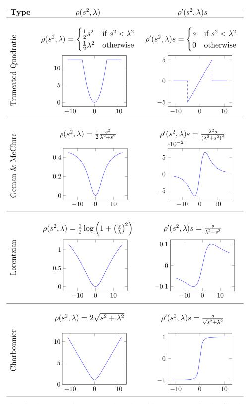
Table 1: Examples of robust error functions. The value of  $\lambda$  is 5, except for the Charbonnier function ( $\lambda = 1$ ). This is a differentiable approximation to the  $L^1$  norm that is typically used in variational optical flow methods, like in [17].
