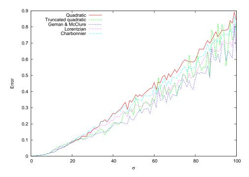
Figure 8: Error evolution,  $\tilde{d}(\mathbf{H}_{gt}\mathbf{x}_i, \mathbf{H}_e\mathbf{x}_i)$ , with respect to Gaussian noise of standard deviation  $\sigma$ . We used the Dimetrodon sequence and a similarity transform.
