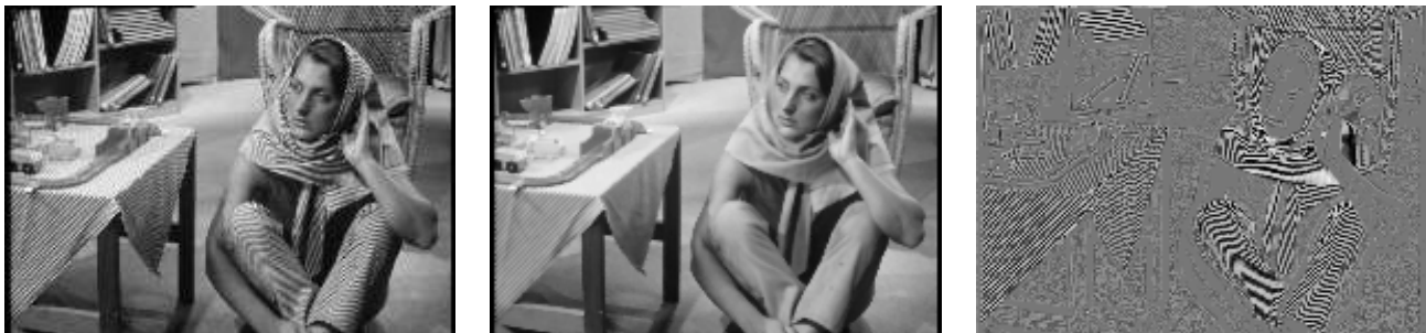
Figure 1: Decomposition of Barbara gray image (left) in cartoon (center) and texture (right). The result was obtained with the non-linear filter pair using L_\sigma ( \sigma = 1.5 ) proposed in [3].
