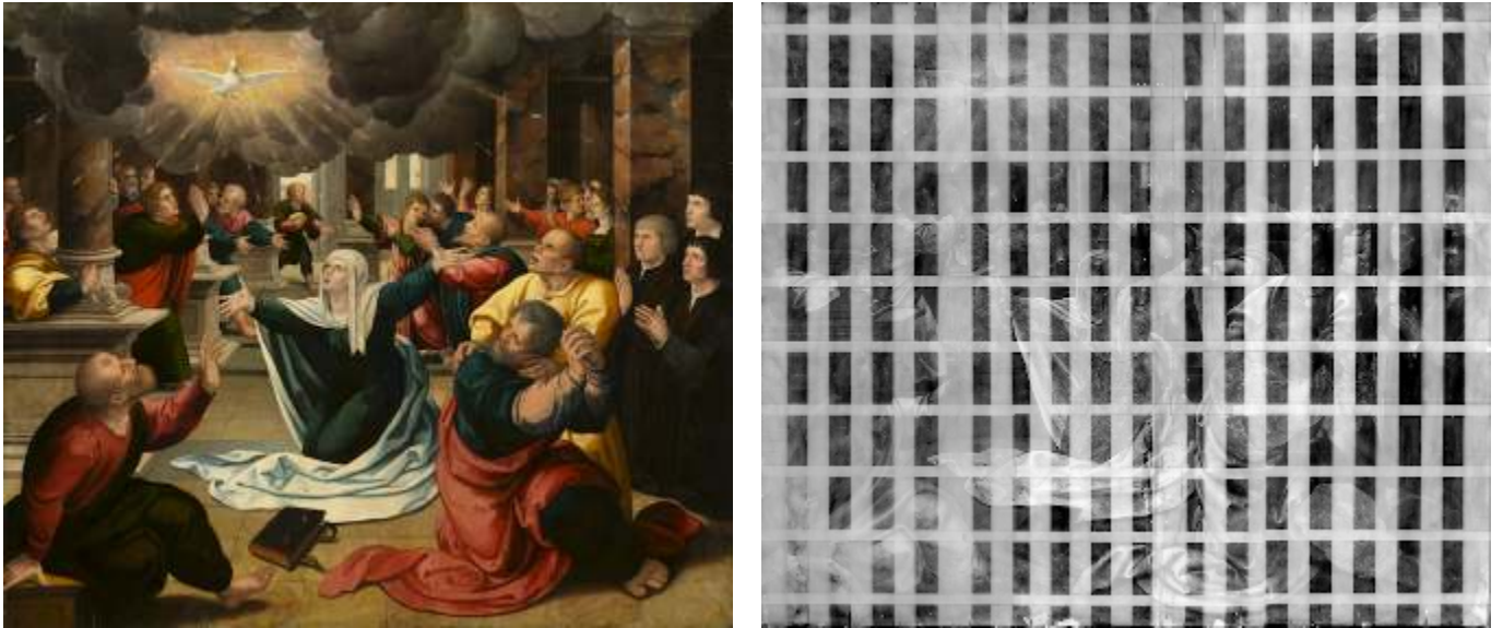
Figure 2: Van Orley's The Pentecost (1525). Left: visual photograph. Right: X-ray image clearly showing the cradle structure.
