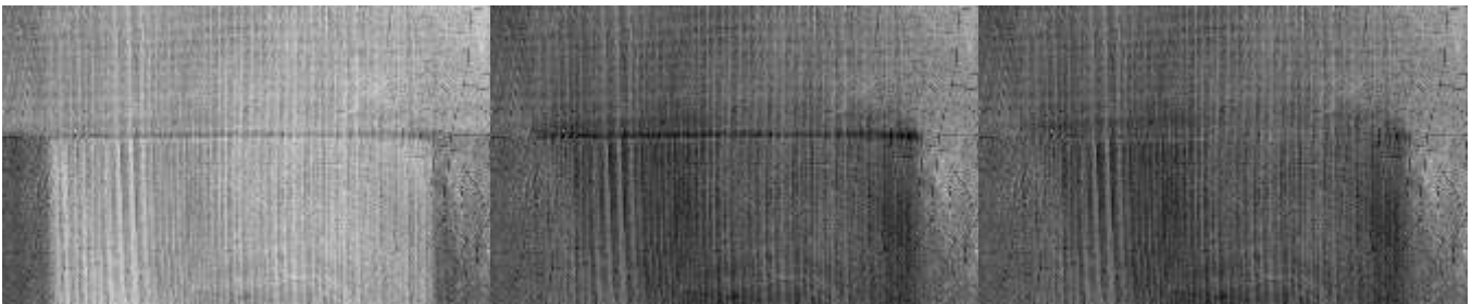
Figure 9: Overcorrection at cross-segments. Left: original X-ray at cross-section. Middle: over-corrected cross-section artifact. Right: cross-section after artifact removal.
