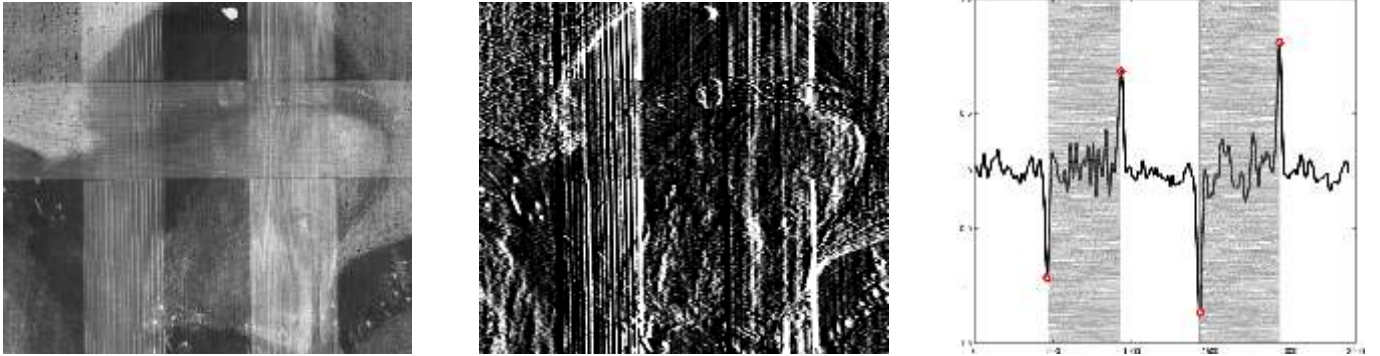
Figure 4: Coarse estimation of cradle segment positions using a horizontal gradient operation. Left: original X-ray. Middle: result after vertical edge detection. Right: plot of edge detection coefficients, summed along the columns and smoothed. Points in red mark the start/end of cradle pieces and gray marking their location.
