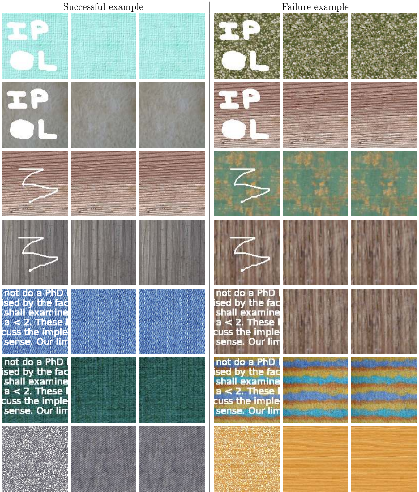
Figure 5: Examples of texture inpainting with k_{\max} = 100 and k_{\max} = 1000 . All images have size 128 \times 128 . Successful examples are presented in the left column while (relative) failure examples are presented in the right column (please zoom in for close inspection).
