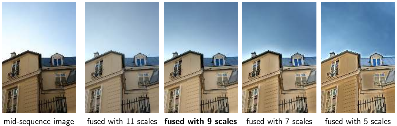
Figure 14: Fusion results with more or fewer scales. For this sequence the algorithm normally uses 9 scales. With more scales the halo disappears but the result loses contrast due to the out-of-range artifact and final normalization. With fewer scales the halo becomes thinner and thus more visible. Parameters: \omega_c = \omega_s = \omega_e = 1 , using robust normalization with 1% of clipping on both white and black sides.
