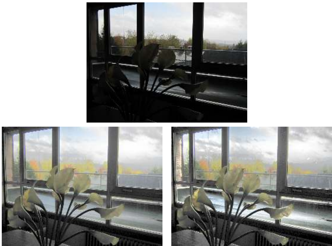
Figure 4: Top: original image. Bottom: Bottom: left, result of classical HE; right, result of MLHE HE (default parameters: L_{\max} = 7 , A_{\min} = 20 , r_{\max} = 3 , r_{\min} = 0.8 ).
